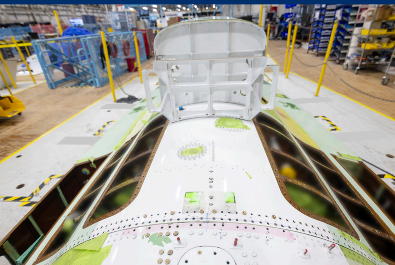
The F-16 Block 70/72 undergoes the critical "mating" process, where the aft fuselage is precisely aligned and attached to the main fuselage, a key step in delivering 21st Century Security® capabilities to global customers.
