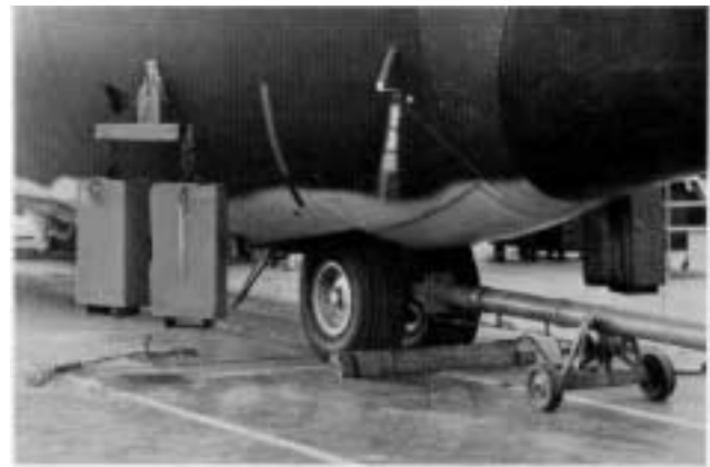
Weights are suspended from jack fittings on the Hercules nose section to stabilize balance during assembly at Lockheed-Georgia.
