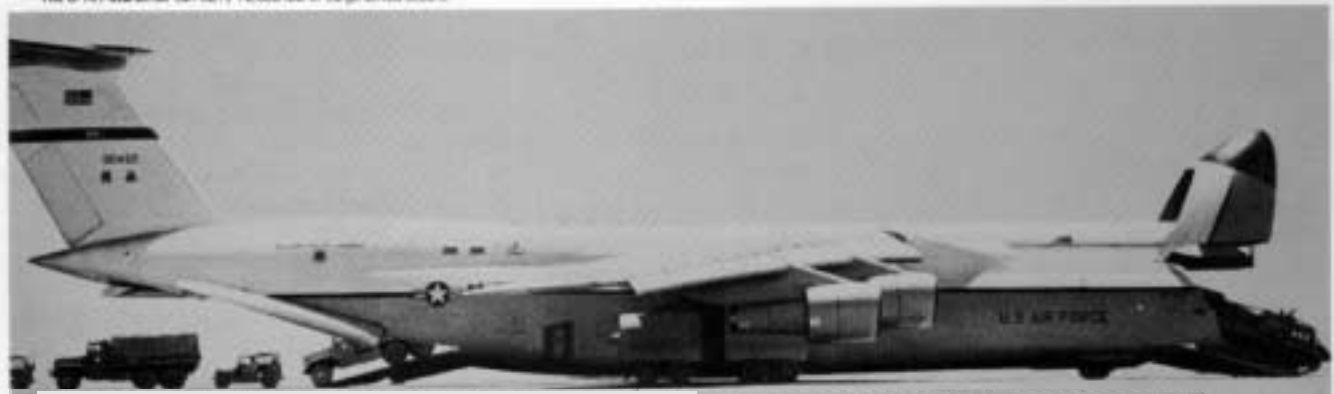
The C-5A Galaxy can carry 220,000 lbs. of anything from giant Chinook helicopters to 5 ton M 60 tanks.
