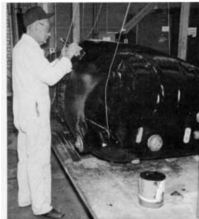
A center cell, bottom up, is receiving a brush coat of blue leak detection compound. White stenciled specifications show through the coating.
