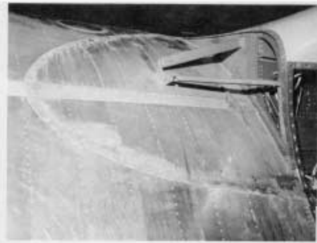
Corrosion from entrapped contaminants in wing fairing.
