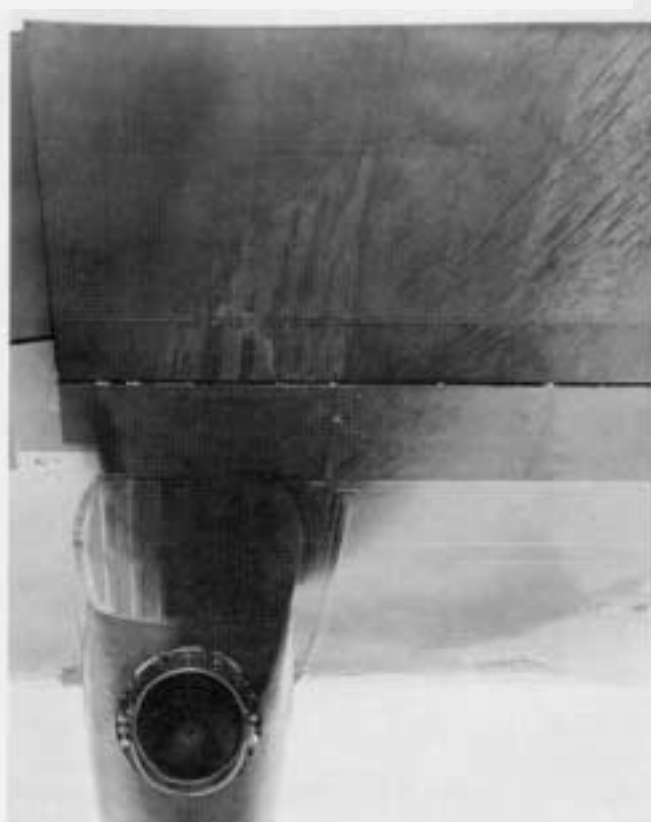
Lower Left: A more frequent cleaning of the engine exhaust trails is necessary in any environment. Upper Right: Drain holes in cargo door skin. Lower Right: A cargo that leaves corrosive deposits.
