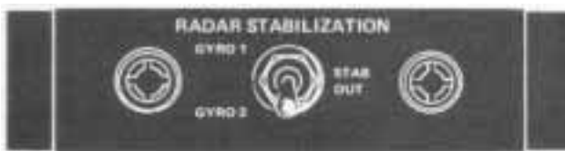
RADAR STABILIZATION CONTROL PANEL
