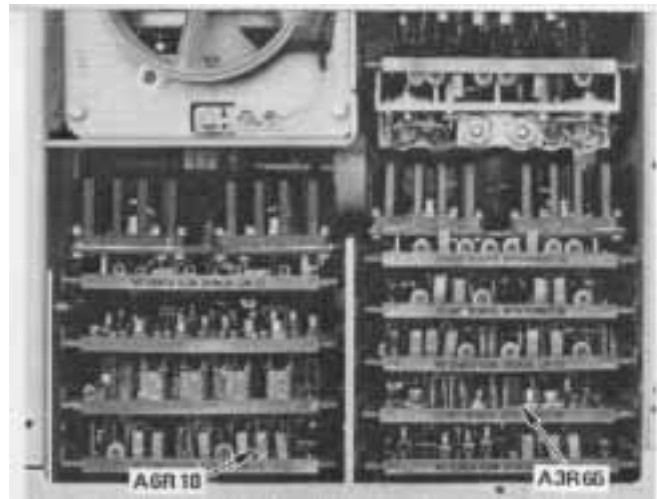
Figure 2. A dash 3 navigator's indicator with cover removed for access to adjustment points. NOTE: Cursor alignment for the dash 3 indicator must be accomplished on the bench while the dash 1 and dash 2 indicators can be adjusted on the airplane. On the dash 1 and dash 2 indicators there will be a potentiometer, A3R65, in the position noted on the photo, which is used to adjust for cursor position.
