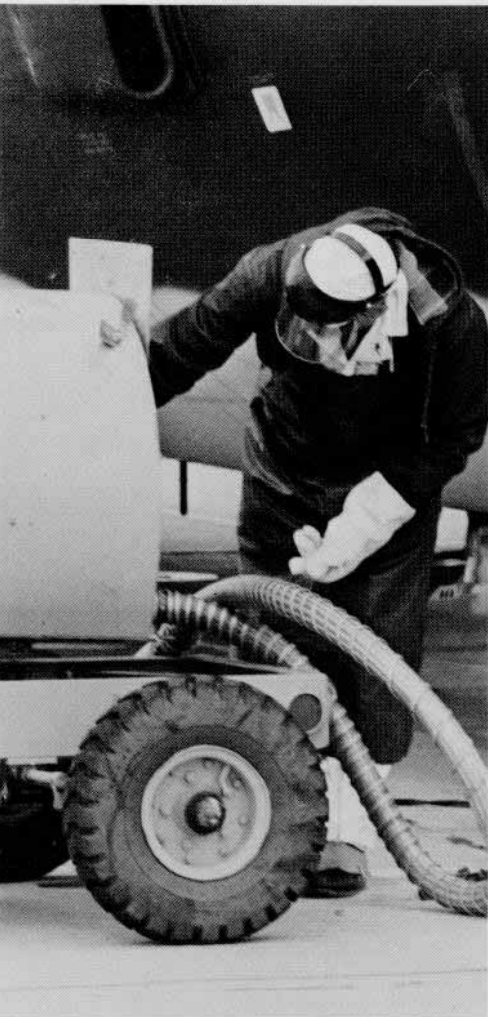
Installing the drain tube between the overboard vent opening and the drip pan.
