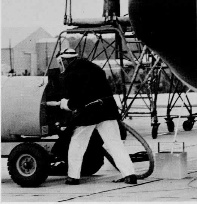
Purging the transfer cart system.
