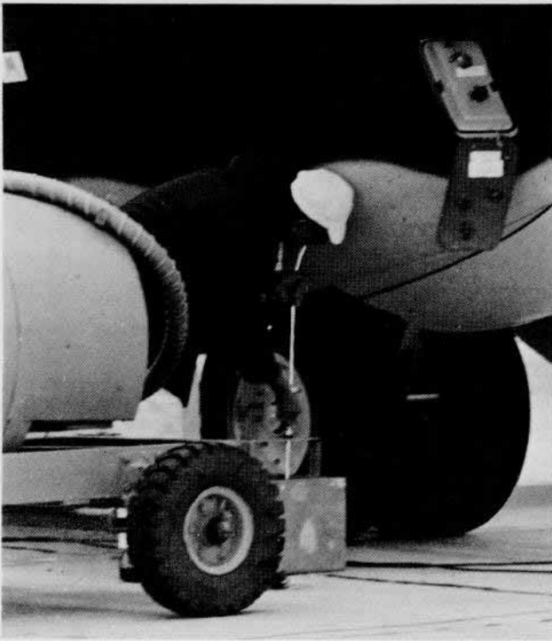
Installing the drain tube between the overboard vent opening and the drip pan.
