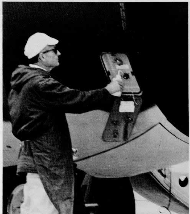
Cleaning hose connection fittings on the service panel.
