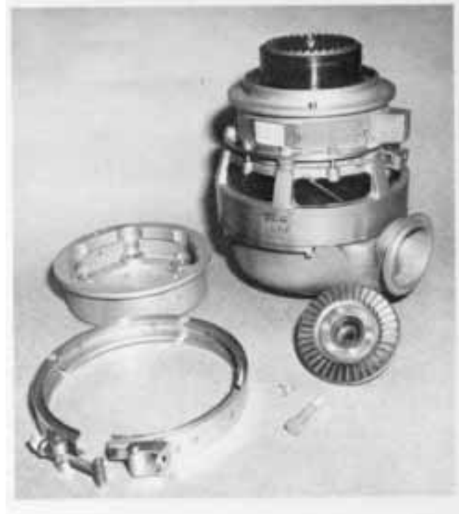
Bendix starter with engine jaw coupling and mounting hardware.
