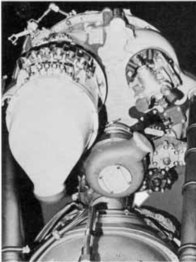
Left: Pneumatic starter location on back of engine reduction gearbox. Above: Starting system components – (1) air control valve (2) pressure sensing line (3) starter (4) speed switch assembly (push button starter controls only).
