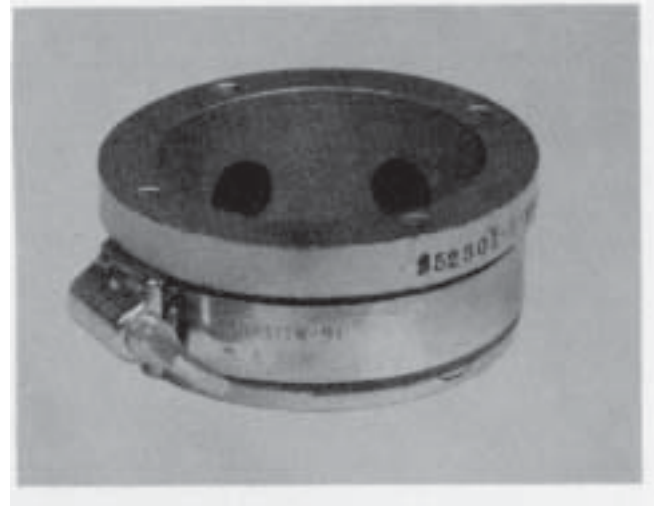
Clamp and tape on older spacers to prevent entry of dirt.
