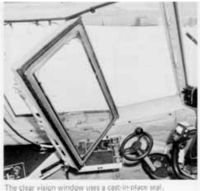
The clear vision window uses a cast-in-place seal.
