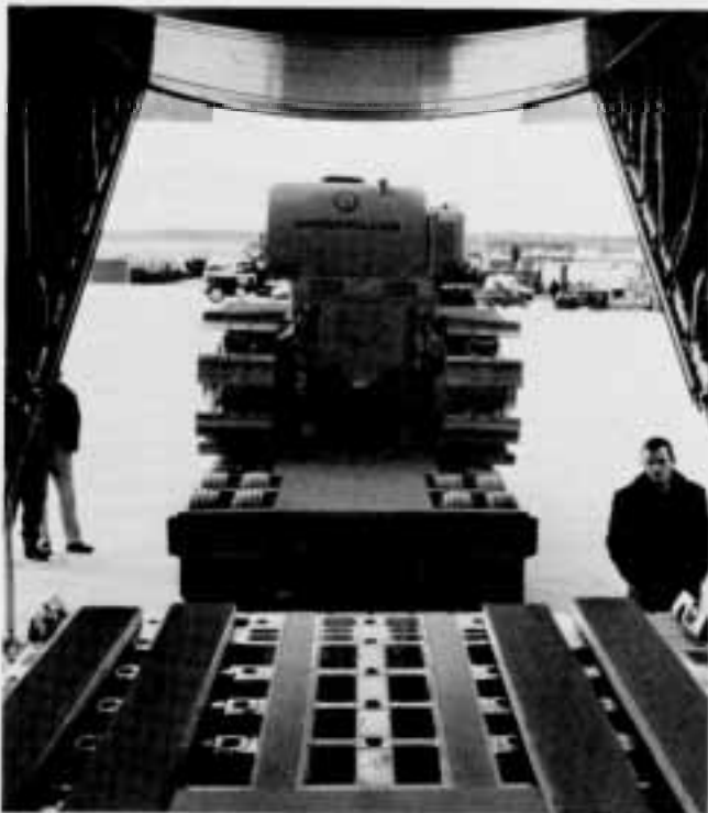
Loading of large machinery and equipment requires special planning for the selection and placement of shoring
