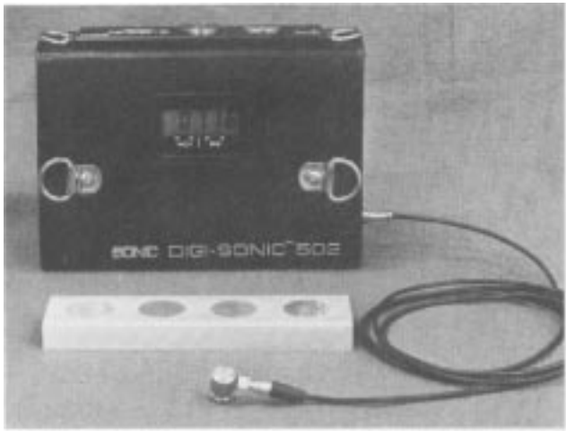
Figure 7. Digi-Sonic 502 ultrasonic test instrument and reference standard.
