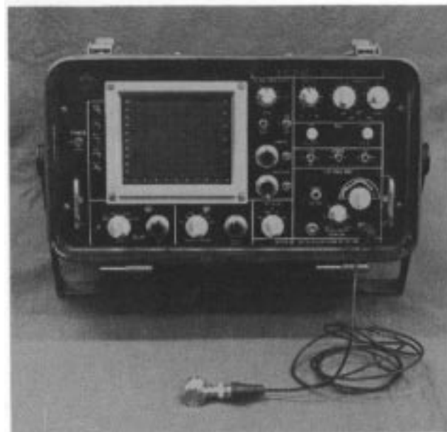
Figure 6. Sonic Mark IV ultrasonic test instrument.
