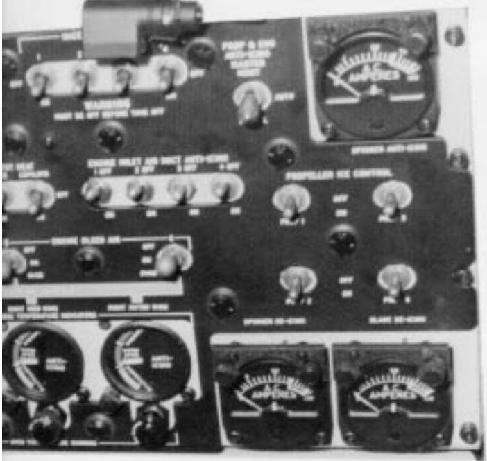
monitored from the anti-icing panel in the flight station.
