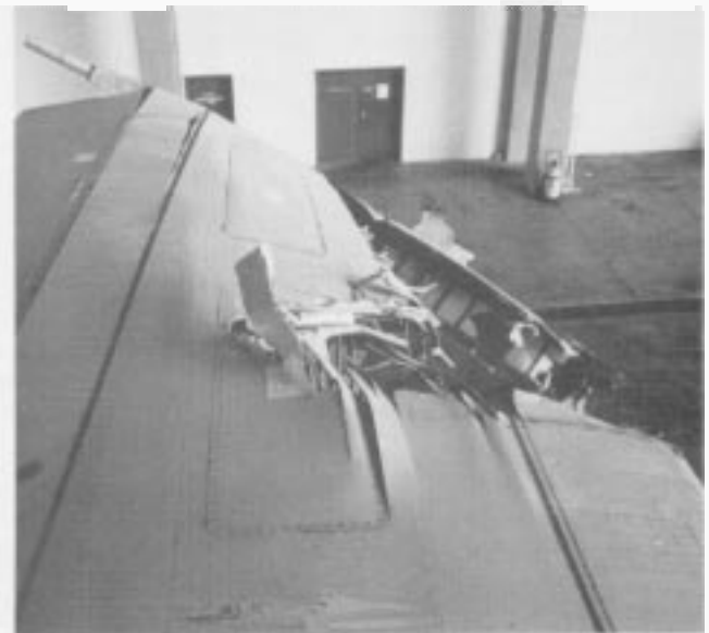
The wing of this airlifter sustained severe damage when it stuck a hangar after the engine-run crew lost control.
