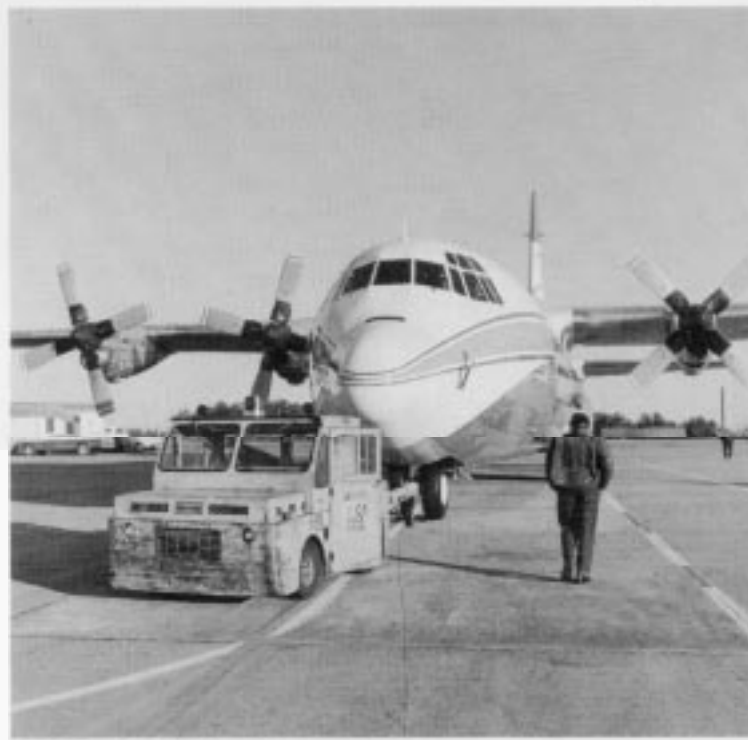
Moving the aircraft in a straight line for two revolutions of the main tires may permit all hooks to engage properly.
