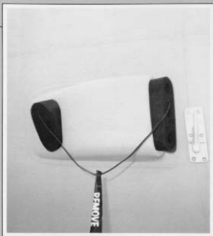
Figure 6. Flight station air conditioning system plug set.
