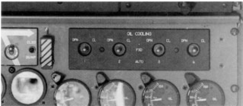
Figure 4. Oil cooling augmentation control panel--recent NVIS-equipped USAF: C-130H aircraft.
