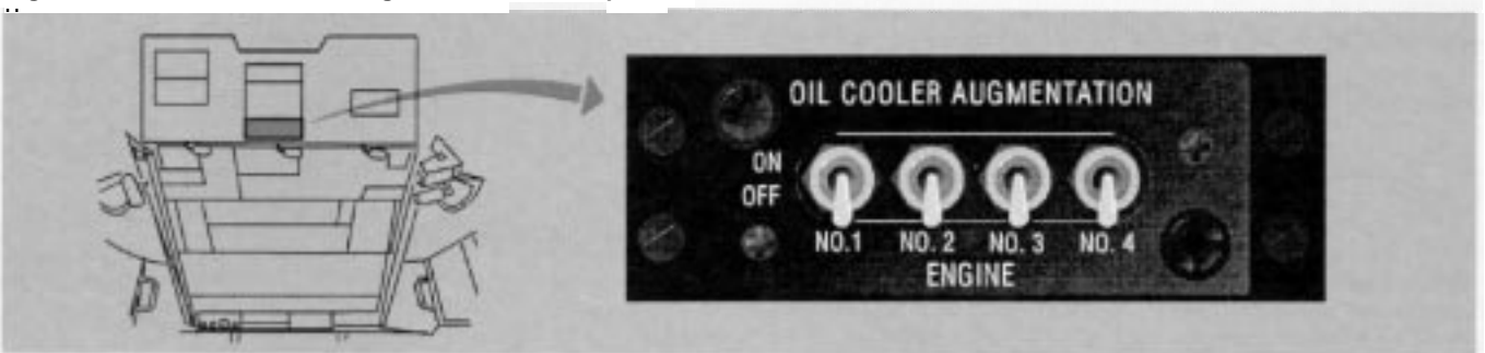
Figure 3. Overhead oil cooler augmentation control panel.
