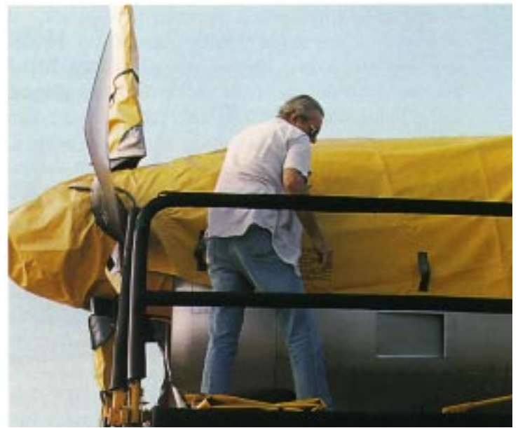
The nacelle cover encloses the nacelle; overlaps the spinner.
