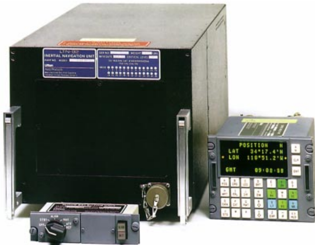
Components of the LTN-92 include the main INU assembly containing laser gyros, power supply, and system electronics; the mode selector (foreground); and the CDU. The CDU features a five-line, 16-character display and expandable function keys.
