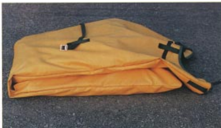
The nacelle cover, spinner cover, and three propeller blade covers will all fit into a single blade cover.
