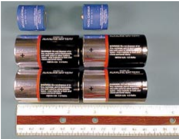
Two small, rechargeable nicads in each unit (top) replace the four heavy, bulky D-cells that power the older EELs.
