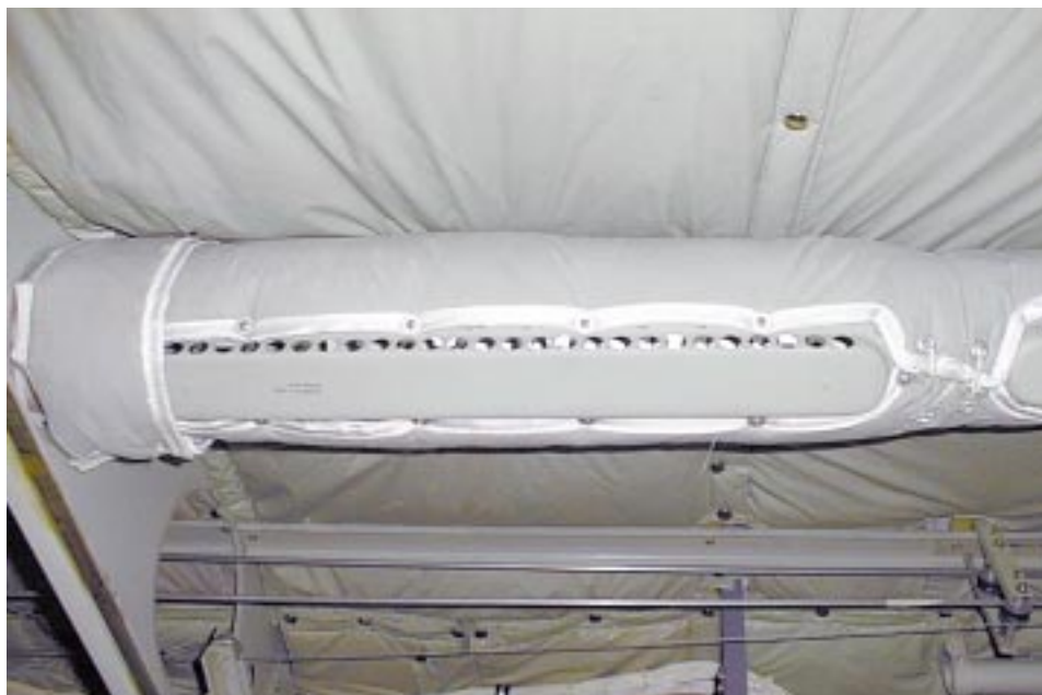
New style cargo compartment heating duct - diffuser directs air to the sides away from the window.
