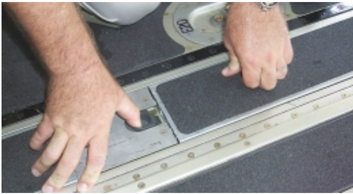
Above and Right: The rollers are easily deployed by releasing the catch and then turning them over.
