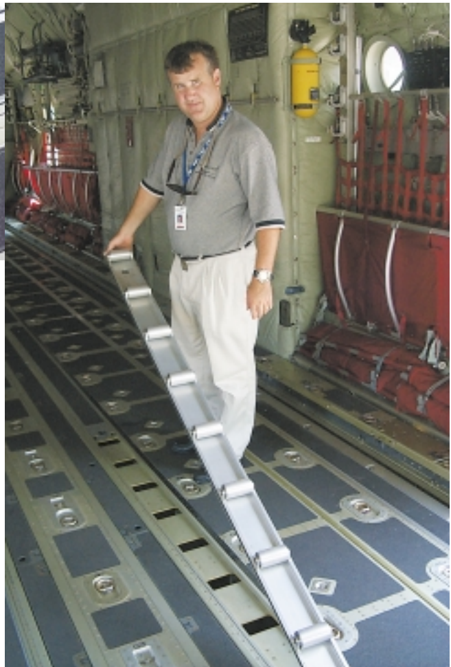
Above and Right: The rollers are easily deployed by releasing the catch and then turning them over.
