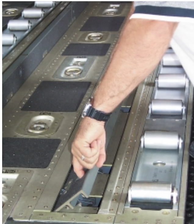
The Center Vertical Restraints are easily deployed as shown above.
