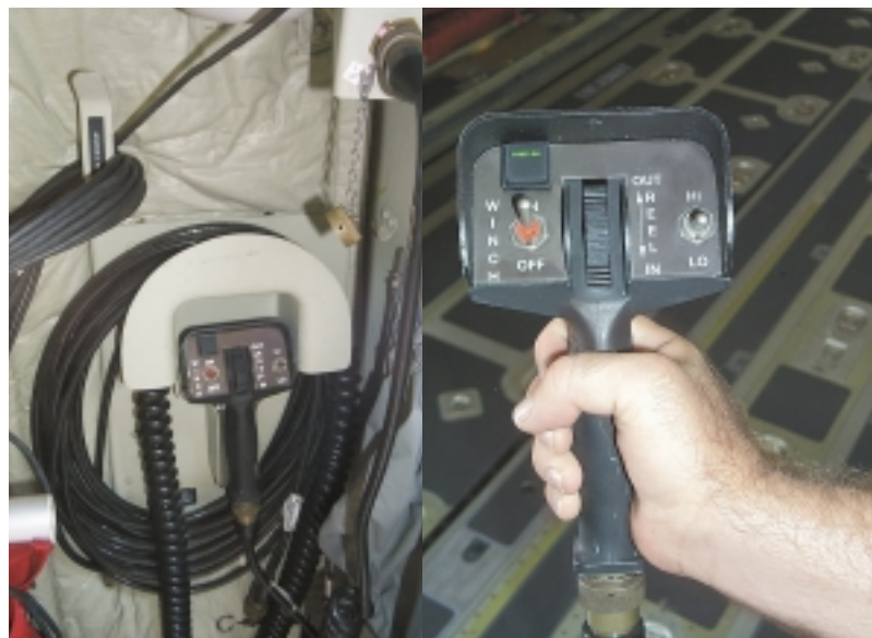
Left: The control pendant for the cargo winch stowed in the forward cargo compartment. Right: Up close photo of the control pendant
