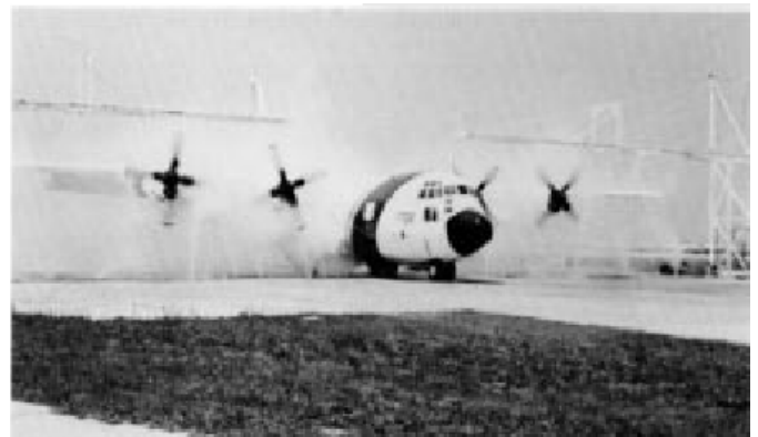
An automated outdoor rinsing facility helps protect Coast Guard aircraft from the corrosive effects of salt spray.
