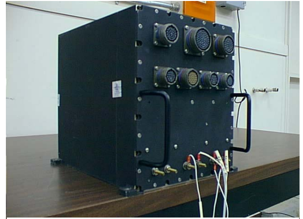
Lighting Control Unit (LCU)
