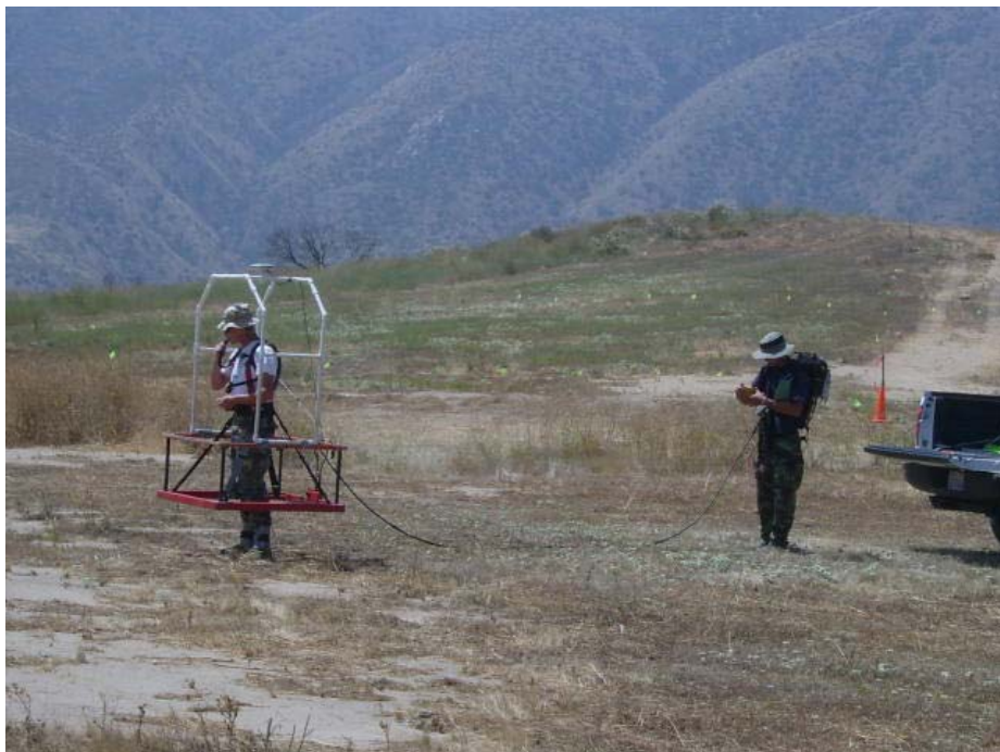
Photo 22: Electromagnetic survey and GPS equipment used to survey areas for possible MEC.
