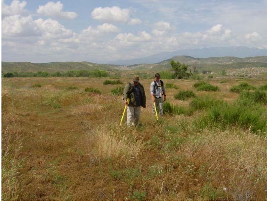
Photo 21: Use of hand held metal detectors to sweep area for metallic objects.
