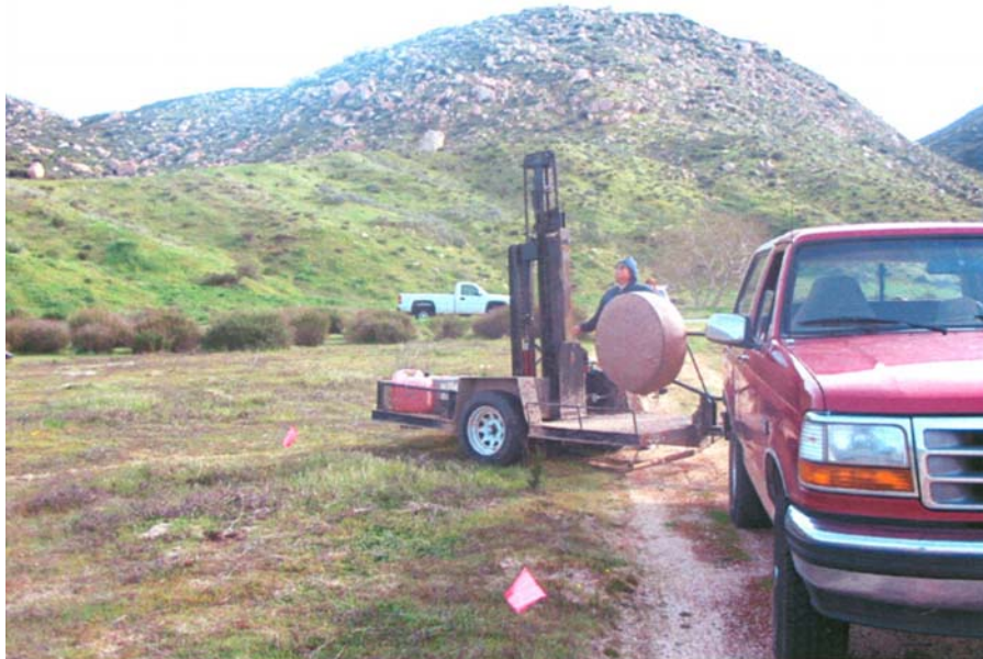
Photo 20: Towable unit used to conduct geophysical seismic studies.
