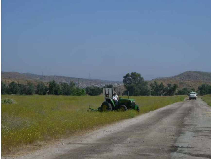
Photo 23: Mower used for site maintenance activities and vegetation clearance prior to conducting MEC surveys. (Note water truck is parked on paved road unless needed for fire response)
