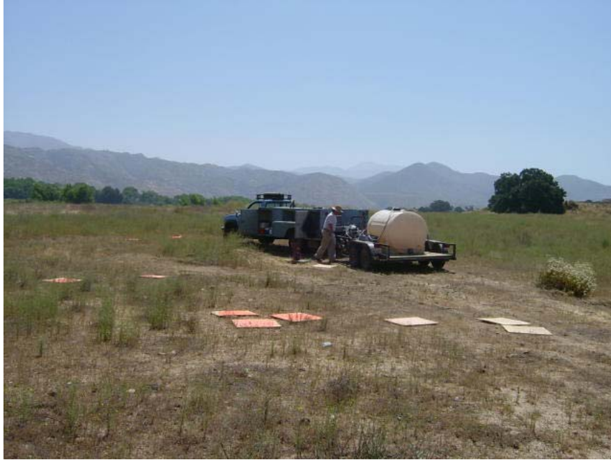
Photo 19: Groundwater sampling truck and trailer (note use of load spreading mats)
