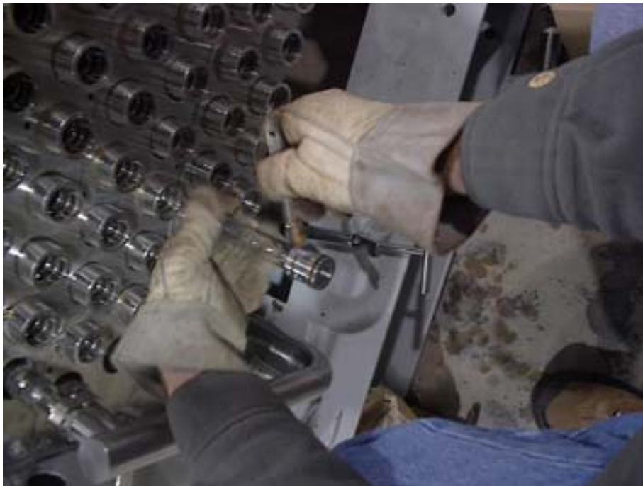
Figure 18: Lubricating Seal Plug O-Rings (Quartz Shown Installed)
