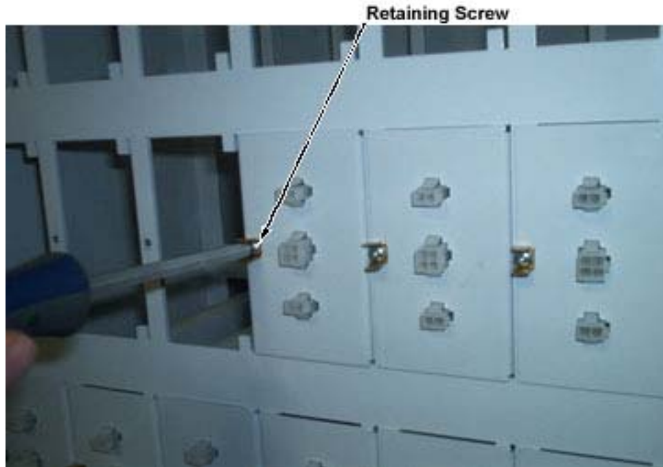
Figure 11: Unscrewing Ballast Card
