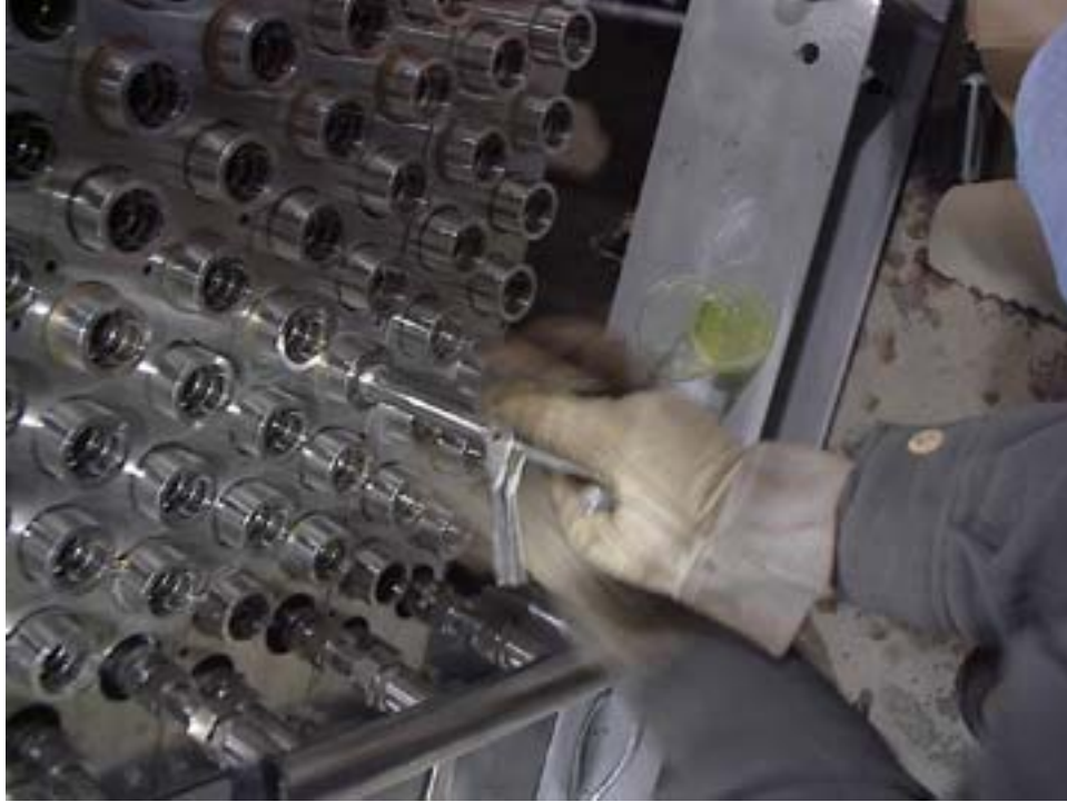
Figure 21: Seating / Unseating Quartz Seal Plug
