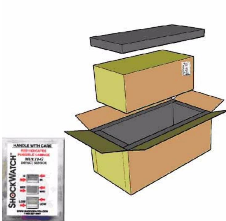
Figure 4. Tri-Axial Shock Watch Multi-G Clip
