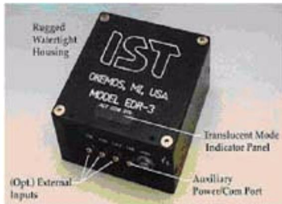
EDR-3C from Instrumented Sensor Technology (IST)
