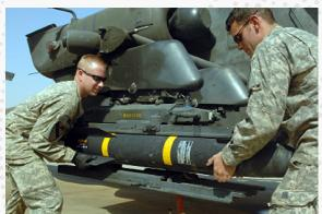
M299 Launcher being loaded with HELLFIRE Missiles.
