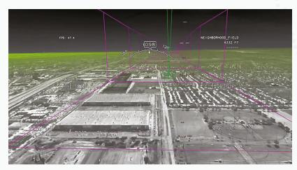
Flight imagery from PDAS' first tactical installation fuses aircraft and DTED data with 360-degree sensor imagery to provide situational awareness and tactical information.
