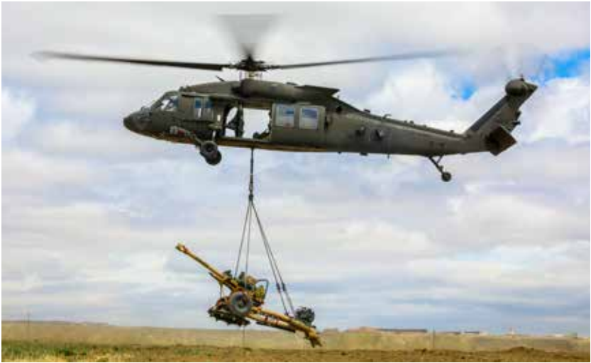
Mission-Ready Cargo Hook Rapid connection of external loads up to 9,000 lbs (4,082 kg)
