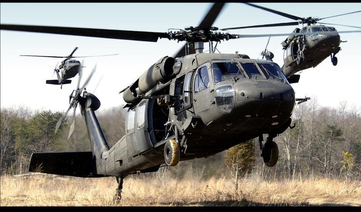
In October 1989, the Black Hawk's engines were upgraded to two General Electric T700-GE-701C 1,890 shp turboshaft engines, and an improved durability gear box was added, resulting in a model designation change from UH-60A to UH-60L. The T700-GE-701C has better high altitude and hot weather performance, greater lifting capacity, and improved corrosion
