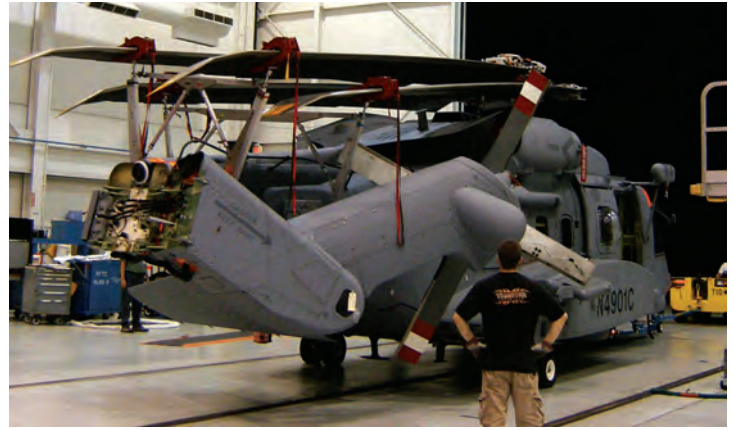
The first prototype CH-148 demonstrated the automatic main rotor and tail folding capabilities. The folding composite tail pylons are built by Kaman's PlasticFab. (Sikorsky photo, December 2009)
