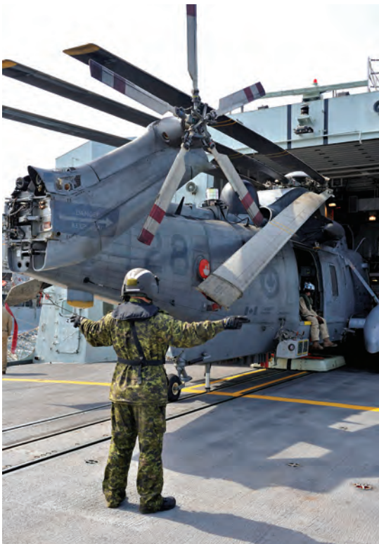
The Helicopter Hauldown Rapid Securing Device (HHRSD) uses a "beartrap" (under the fuselage) to winch in the aircraft and grab the main probe; the tail probe guides the aircraft along the track. (Dept. of National Defence photo, September 2012)
