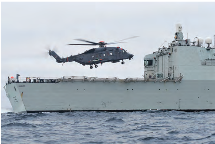
A second round of Ship Helicopter Operating Limitations (SHOL) trials took place on the HMCS Montreal with the CH-148 prototype during 42 days at sea in January-February 2011. (Sikorsky photo, February 2011)
