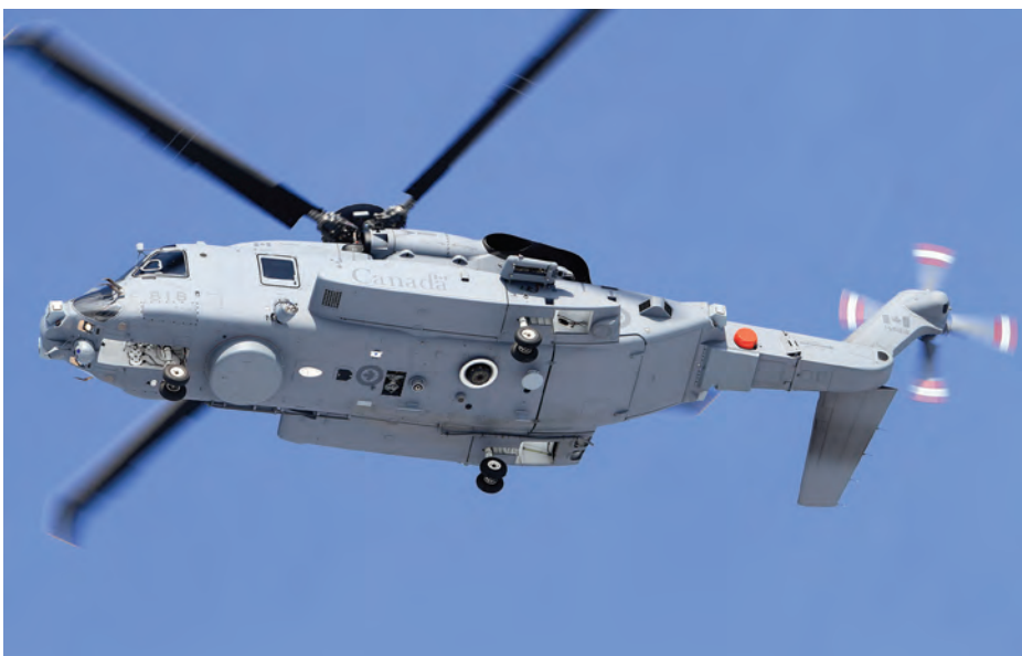
From tip to tail, the most obvious underside features in this photo are the FLIR, OceanEye radar, sonobuoy chute, cargo hook, C-RAST probe, dipping sonar (off axis), antenna, rear ramp and tail fold. (Photo © Michael Durning, used with permission, March 2015)
