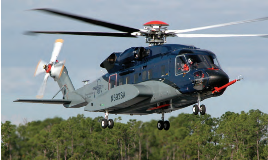
The fifth S-92A was modified as a prototype fly-by-wire S-92F, with first flight on Dec. 20, 2007. (Sikorsky photo)
