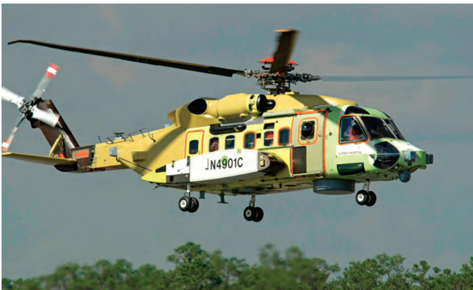
The first CH-148 (No. 148801) made its initial flight on Nov. 15, 2008. The unpainted aircraft highlights the composite self-folding tail structure. (Sikorsky photo)
