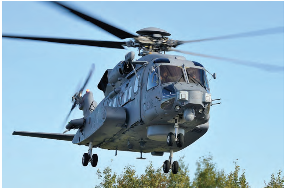
In this photo of the first official training flight in Oct. 2013 at Shearwater, the square missile approach warning systems on either the nose are evident, with the round ESM sensors below them. The FLIR ball is just ahead of the nose gear, facing rearward for protection. The winch and sponson-mounted torpedo rack are also clearly visible. (DND photo)
